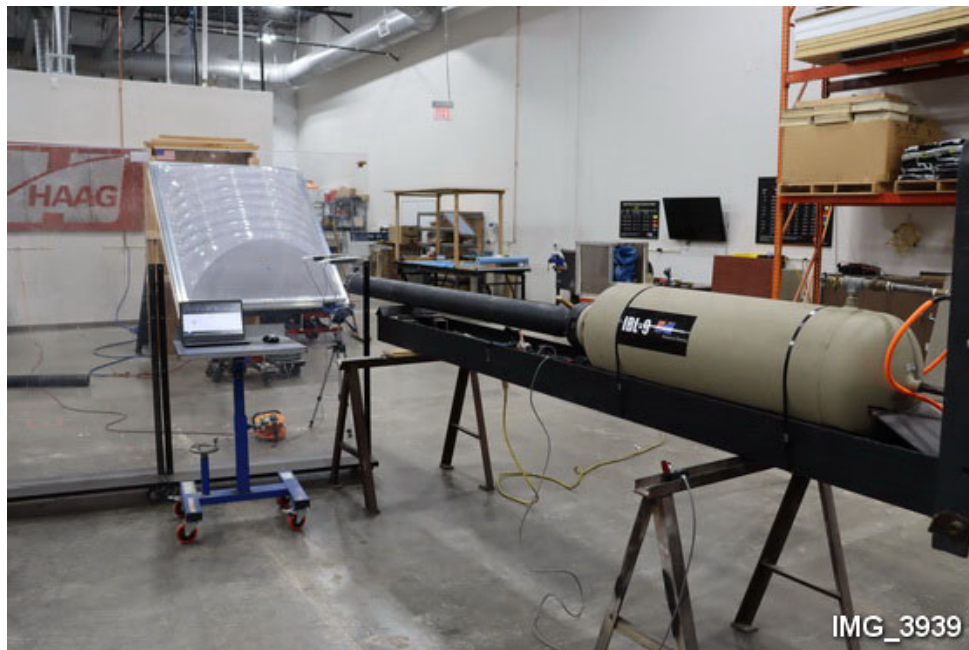
D1. Overview of test setup with Haag IBL-9 ice ball launcher.
