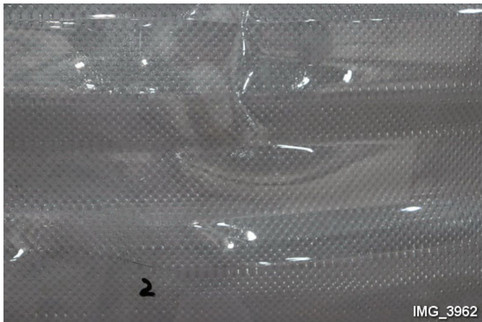
D6. Overview of Impact 2 with 4 inch ice ball. (Note impact caused dent and buckle.)
