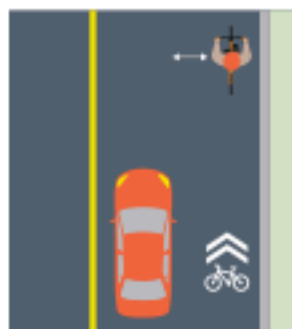
Example of shared roadway. Three (3) feet of distance must be maintained between the car and cyclist.
