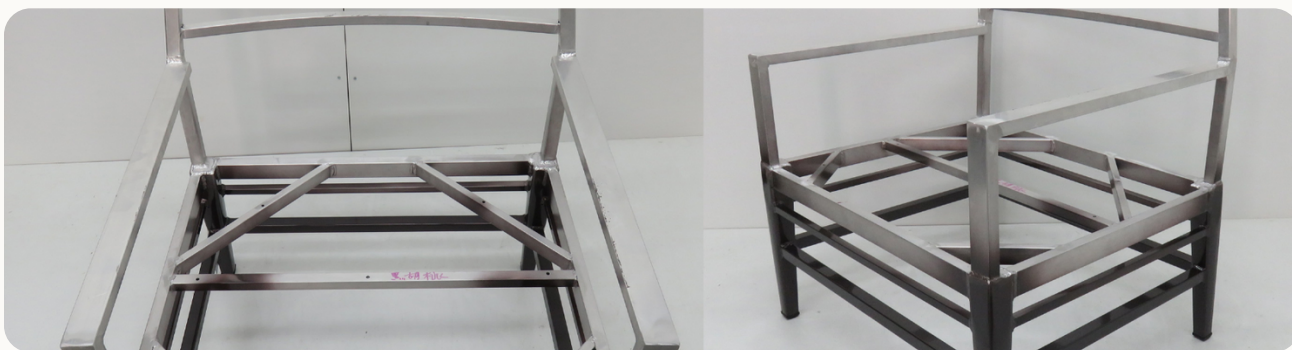
The fully welded aluminum frame before upholstery.
