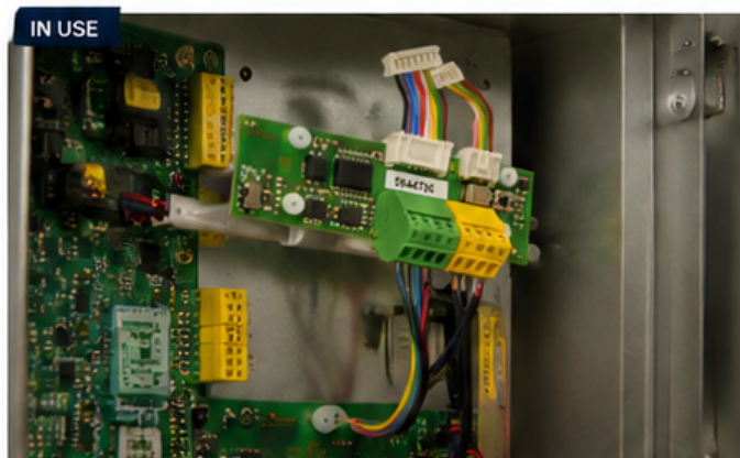
Mounted inside a FEIG controller. Provides additional RS485 and CAN connectivity.
