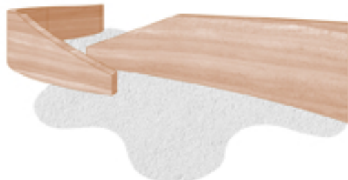
5. Rammed earth curved walls
