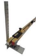
Platform Rail Gauges
