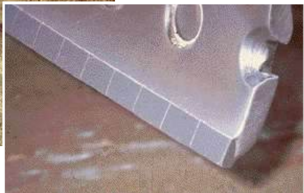
An example of a carbide-faced blade after 650 hours of use. The center sections had been exchanged with the outer sections once during this time.
