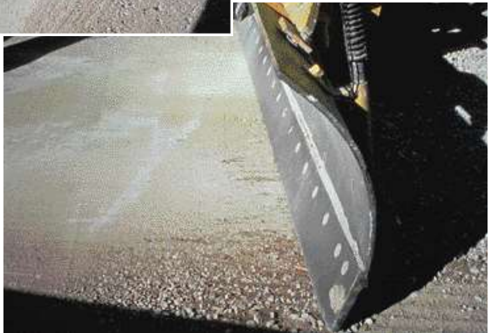
The technique of backdragging can save time.
