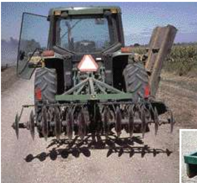
A small rear-mounted tandem disk on a mower tractor.
