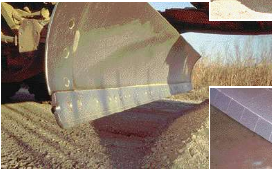
An example of a carbide-faced blade after 650 hours of use. The center sections had been exchanged with the outer sections once during this time.
