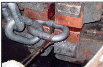
Figure 12 – Correct position of chain link in copper jaws
