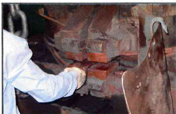
Figure 11 – Good condition of flash butt welding copper jaws
