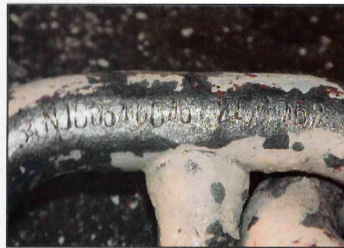
Figure 23 - Example of incorrect LR stamp and incorrect stamp location.
