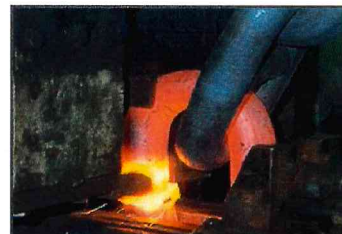
Figure 14 – Machine removal of the extruded flash
