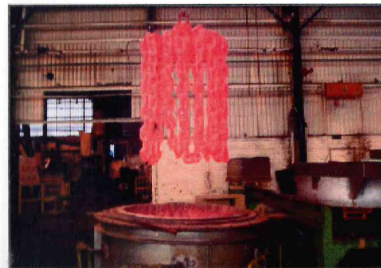
Figure 18 – An example of chain correctly fixtured for batch heat treatment
