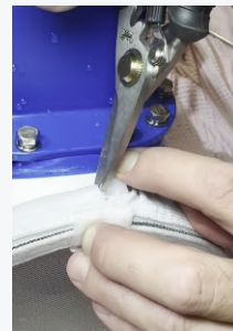
CUT OLD SECURING TIE
